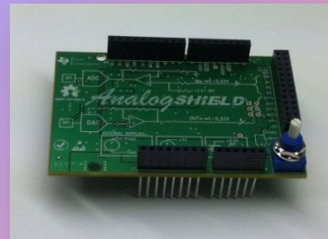
Analog shield for the Arduino platform – includes ADC, DAC, power supplies
